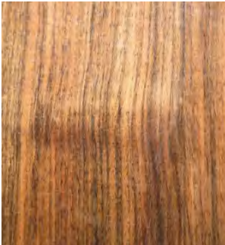
▲ Pic.17 Walnut is a beautiful timber with rich colour streaks and a crisp grain, excellent for fine shaping
